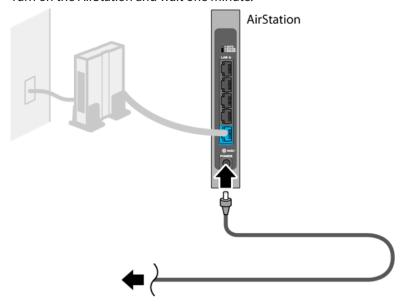
If using a wired LAN, connect the AirStation LAN port and computer using a LAN cable. If using a wireless LAN, connect the computer to the wireless LAN as described in chapter 4.
